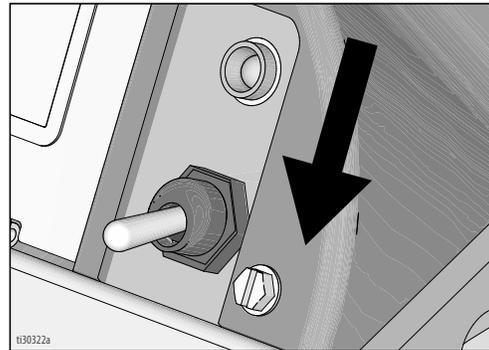
3. Plug charging cord into charging port on the unit. Connect an extension cord, minimum 12AWG (2.5mm<sup>2</sup>), to the charging cord and plug it into wall power.
