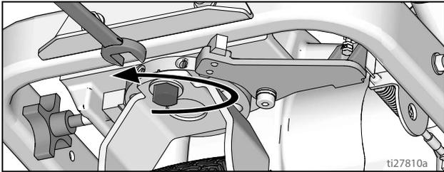
2. If striper arcs to the right, loosen left set screw and tighten right set screw for fine tune adjustment.
