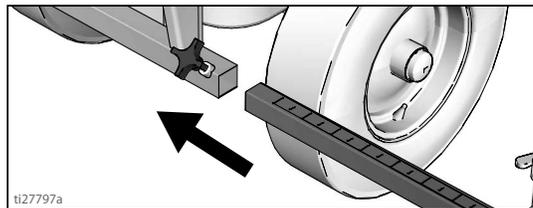
4. Tighten gun arm knob into gun arm mounting slot.
