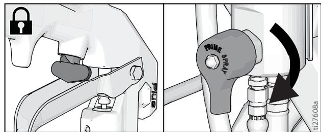
5. If you suspect the spray tip or hose is clogged or that pressure has not been fully relieved:
