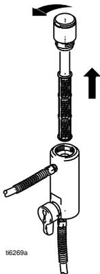
4. Clean filter, guard and SwitchTip in flushing fluid.
