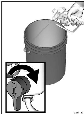
9. Turn pressure control to Fast Flush (ES 1000), or 1/2 position (ES 2000), and operate until the pump runs steady and flushing fluid appears in the waste pail.
