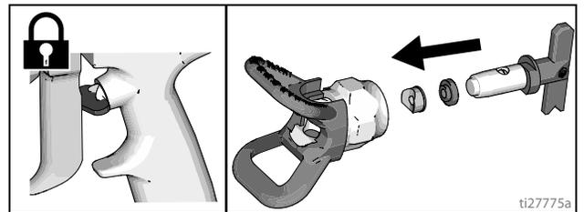
2. Insert SwitchTip in tip bore and firmly thread assembly onto gun.
