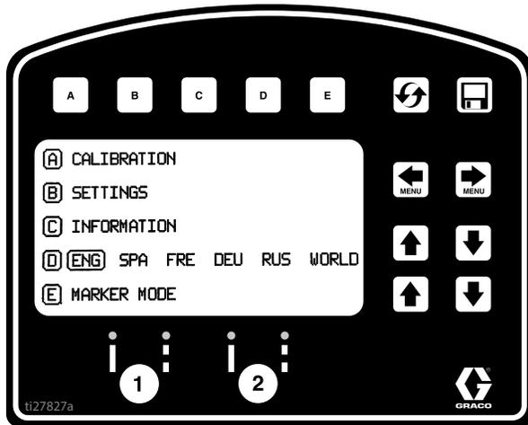
4. Press **A** for Calibration. Set TRAVEL DIST to 25 ft (7.6m) or longer. Longer distances ensure better accuracy, depending on conditions.
