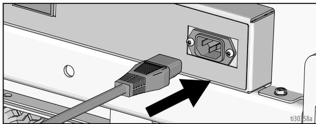
4. When power is connected the voltmeter will turn on and the charger will immediately begin charging. User should be able to see voltmeter start to climb to indicate charging is occurring.
