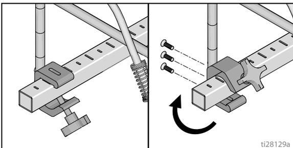
Another option can be to swing the gun out at an angle and rotate the tip guard. This results in better visibility for the user.
