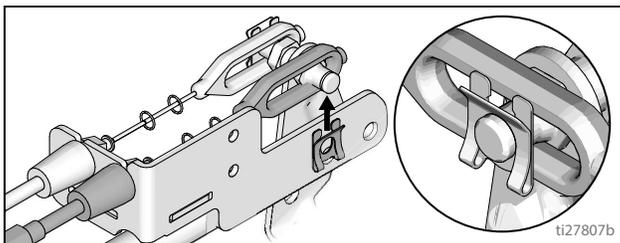
5. Route cable around unit and up through cable holes behind hose mount.
