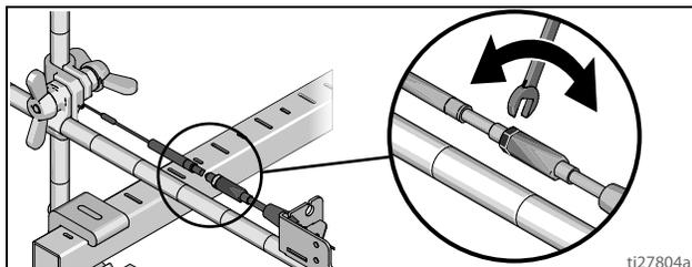
2. Loosen or tighten adjuster until desired result is achieved. **NOTE:** More thread exposed means less gap between gun trigger and trigger plate.
