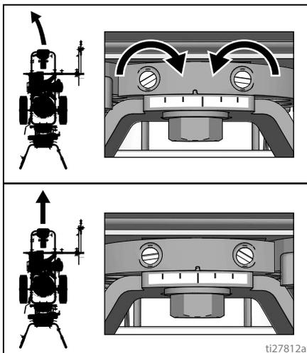
4. Roll the striper. Repeat steps 2 and 3 until striper rolls straight. Tighten bolt on wheel alignment plate to lock the new wheel setting.
