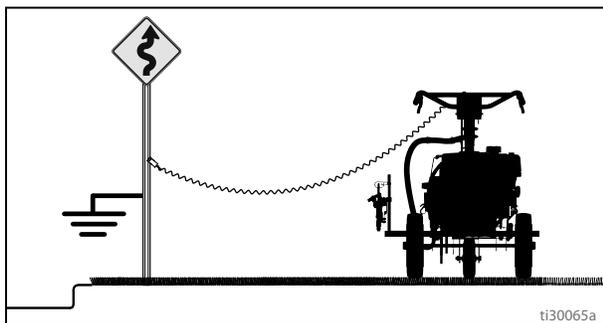
A metal sign post can be used as a true earth ground. Connect the grounding wire and clamp to a metal post. A properly grounded electrical outlet can also be used as a true earth ground. Use the provided adapter.
