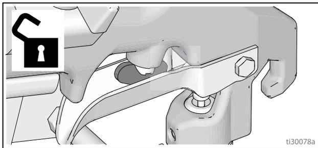
2. Engage gun trigger lock, return SwitchTip to original position, disengage gun trigger lock and continue spraying.
