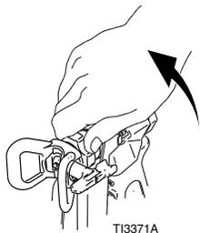
3. Unscrew cap, remove filter. Assemble without filter.
