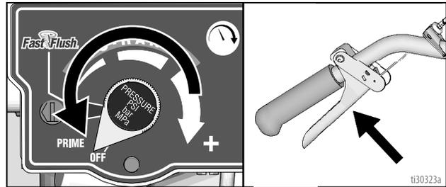
4. Engage all gun trigger locks. Turn prime valve down.
