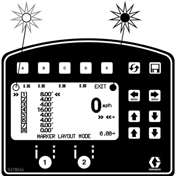
2. Use arrow keys to set up a marker pattern.
