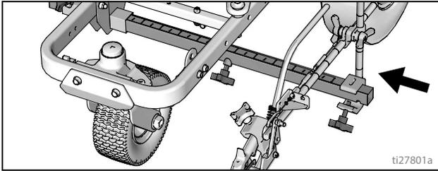
**NOTE:** Make sure all hoses, cables, and wires are properly routed through brackets.
