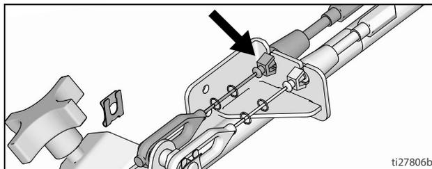
4. Install cable end onto trigger plate pin and install clip.
