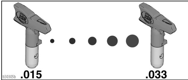
2. Trigger gun and spray test pattern. Slowly adjust pressure to eliminate heavy edges. Use smaller tip size if pressure adjustment can not eliminate heavy edges.
