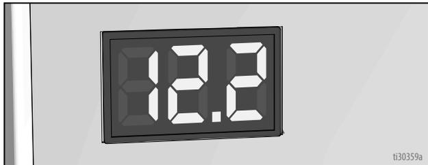
5. Battery will charge to 14.6-14.8 volts and then it will come back down to ~13.6 volts when fully charged.
