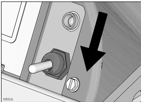
3. Turn prime valve down. Turn pressure control counterclockwise to lowest pressure.
