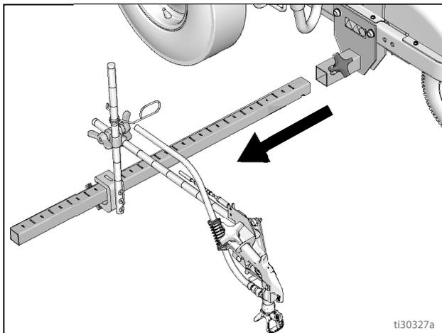
3. Slide gun arm assembly into desired gun arm mounting slot.
