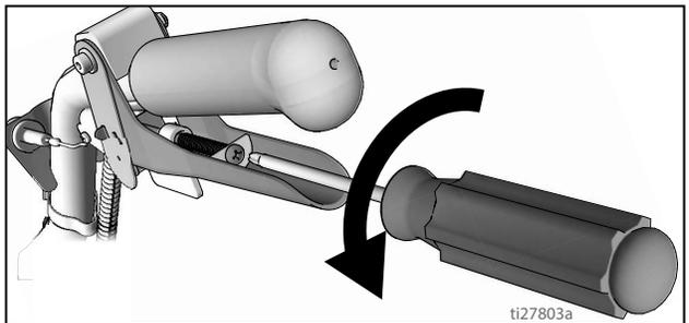
4. Continue adjusting screw in handle until timing of spray icon and fluid spray are synchronized. Adjustment of the gun cables might be necessary.
