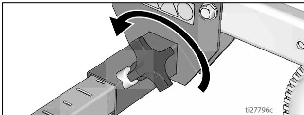
2. Slide gun arm assembly (including gun and hoses) out from gun arm mounting slot.
