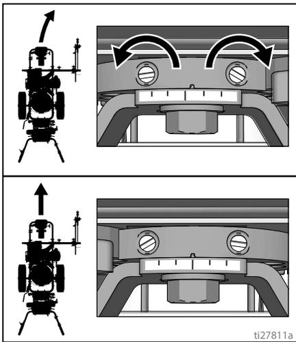
3. If striper arcs to the left, loosen right set screw and tighten left set screw.
