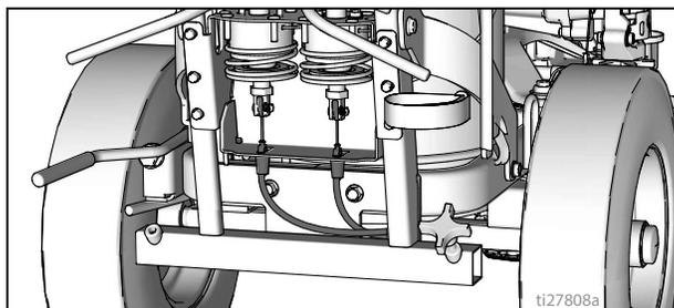
6. Route cable end loop through rectangular hole in bracket and insert plastic cable retainer into the actuator bracket. Install cable end onto actuator rod and install pin.
