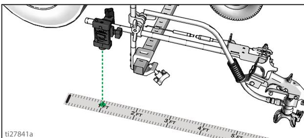
6. Press and release gun trigger control to start calibration.
