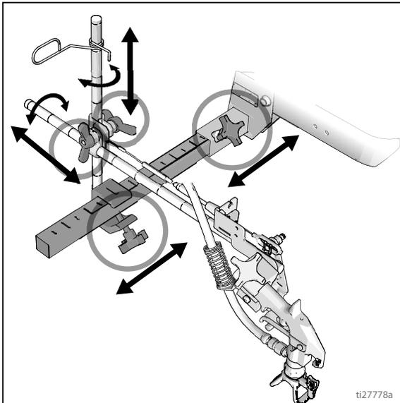
**NOTE:** When striping above a curb, the mounting clamp can be rotated for clearance.
