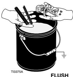
5. Attach ground wire to true earth ground or plug unit into grounded outlet.
