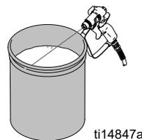
7. Turn prime valve down to DRAIN position and allow flushing fluid to circulate until flushing fluid appears clear.
