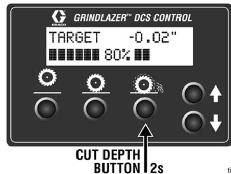
The DCS Control is now ready to grind/scarify. Long press down on the Handlebar Rocker Switch to lower the drum to your Cut Depth Target. Short press up or down on the switch to adjust your Cut Depth on the fly. When finished with your cut, long press up on the switch to raise the drum to the Home position.
