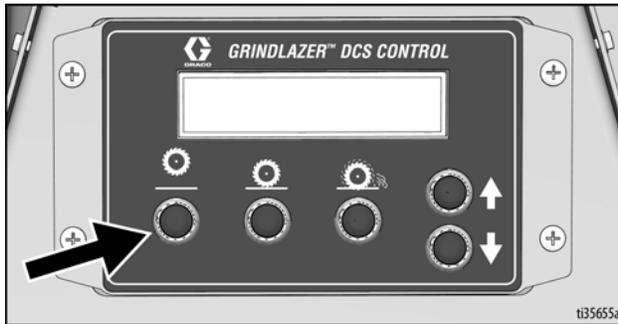
6. **25M994 Model Only:** Make sure Power Switch (B) is in UP position.
