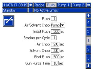
Figure 59 Flush Screen with pump air/solvent chop
