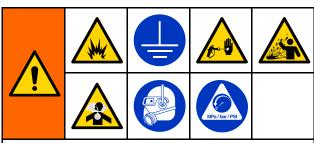
To avoid fire and explosion, always ground equipment and waste container. To avoid injury from splashing, always flush at lowest possible pressure.
