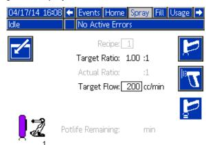
Figure 23 Spray Screen, in Idle Mode
