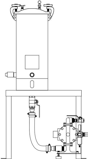
*5 Gallon Tank with Diaphragm Pump and Stand*
