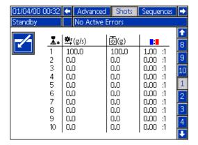
This screen allows the user to edit shot definitions. The contents of this screen change based on the Dispense Mode. Shots may be defined by flow rate and by time (duration), volume, or weight depending on the Dispense Mode selection. See **System #1** on page 64 for Dispense Mode options.
