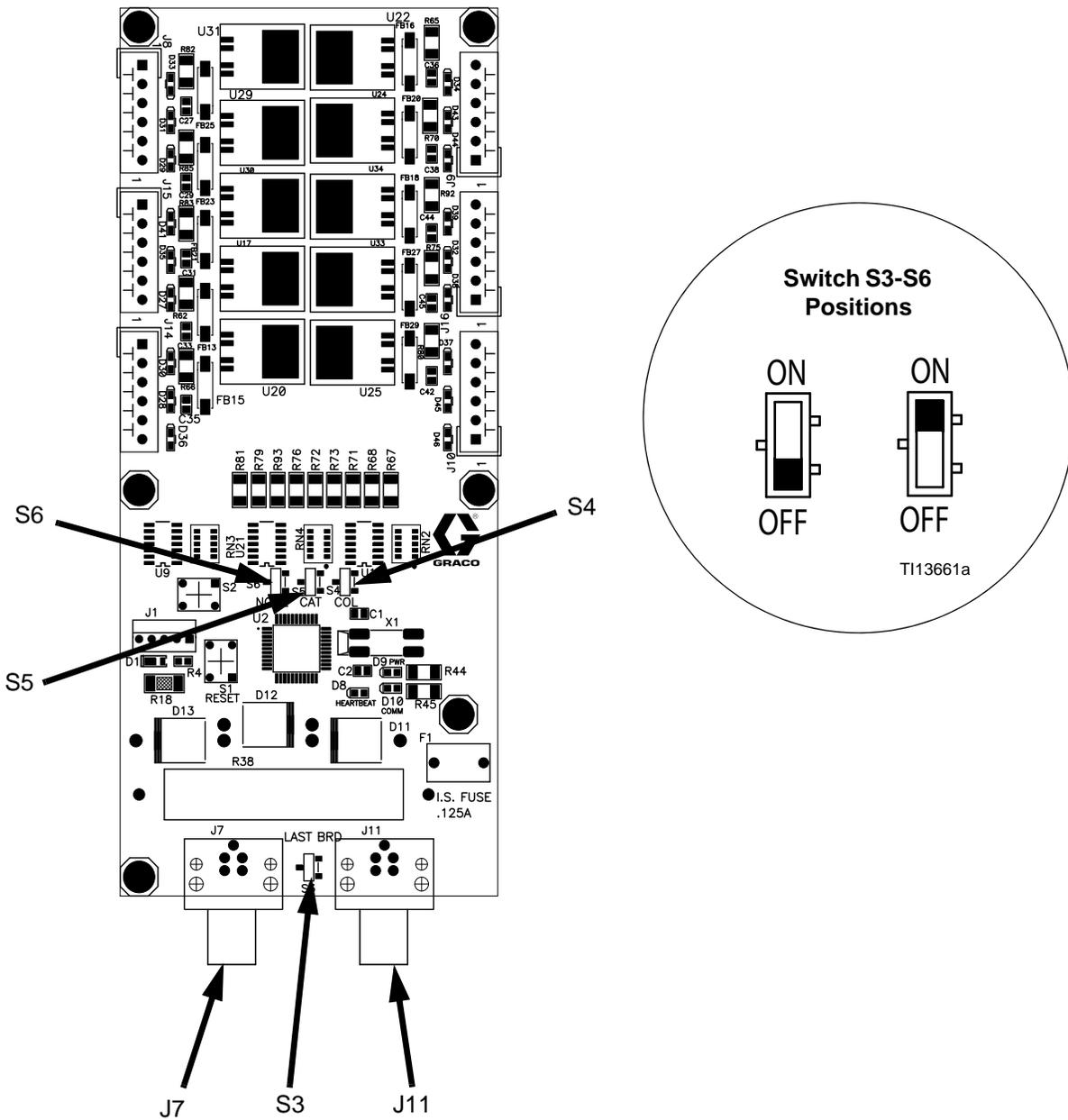
FIG. 21. Color Change Board Switches S3-S6
