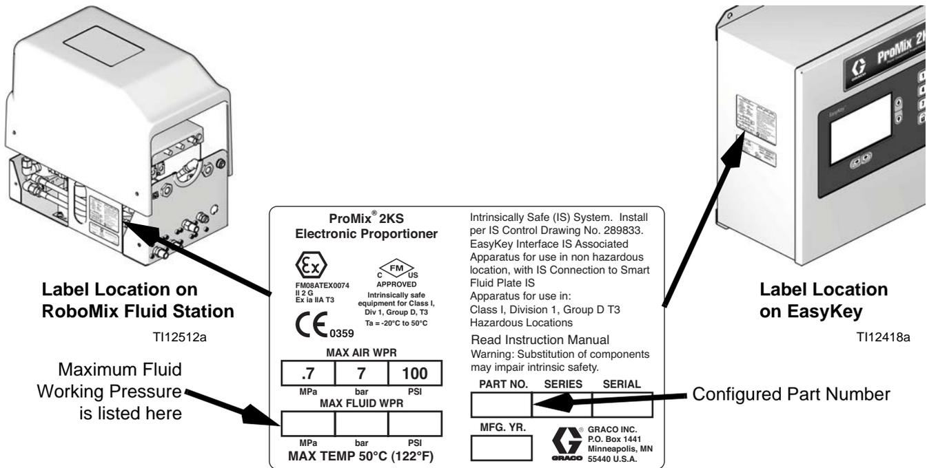
FIG. 2: Identification Label, RoboMix Fluid Station Systems
