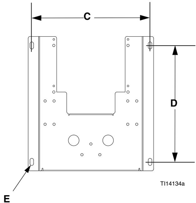
**NOTE:** Height is shown from top of panel to fluid shutoff valves, and does not include the effect of variable fluid integrator heights. Width of panel does not include optional color/catalyst valve stacks.
