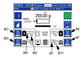
The Tank Fluid Temperature Setpoint (BR), Tank Fluid Temperature (BS), Hose Heater Temperature (BT1), and Hose Heater Temperature Setpoint (BT) display the status of the each of the options. To turn the Tank Blanket Heaters or Hose Heaters on or off, press the Tank or Hose Heater On/Off button (BC, BD, BE, BF). See **Heat Options, Screen #2** on page 29 for more information on temperature control setup.
