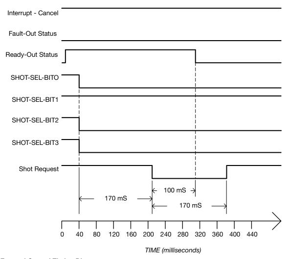
Fig. 39: External Control Timing Diagram
