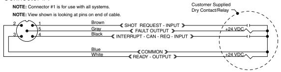
Fig. 37: External Control Interface Electrical Diagram
