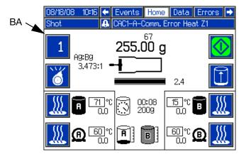
This procedure can be used to initiate auto-refill if Manual Auto-Refill, High Level Auto-Refill, Empty Auto-Refill, or Accumulator mode is enabled. See **Fluid Options, Screen #1** on page 27 for a description of each Auto-Refill mode.
