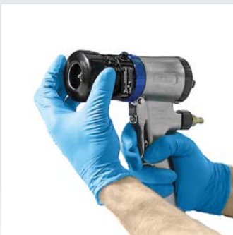
Remove the aircap and retaining ring
