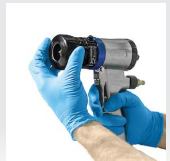
Install the retaining ring and aircap
